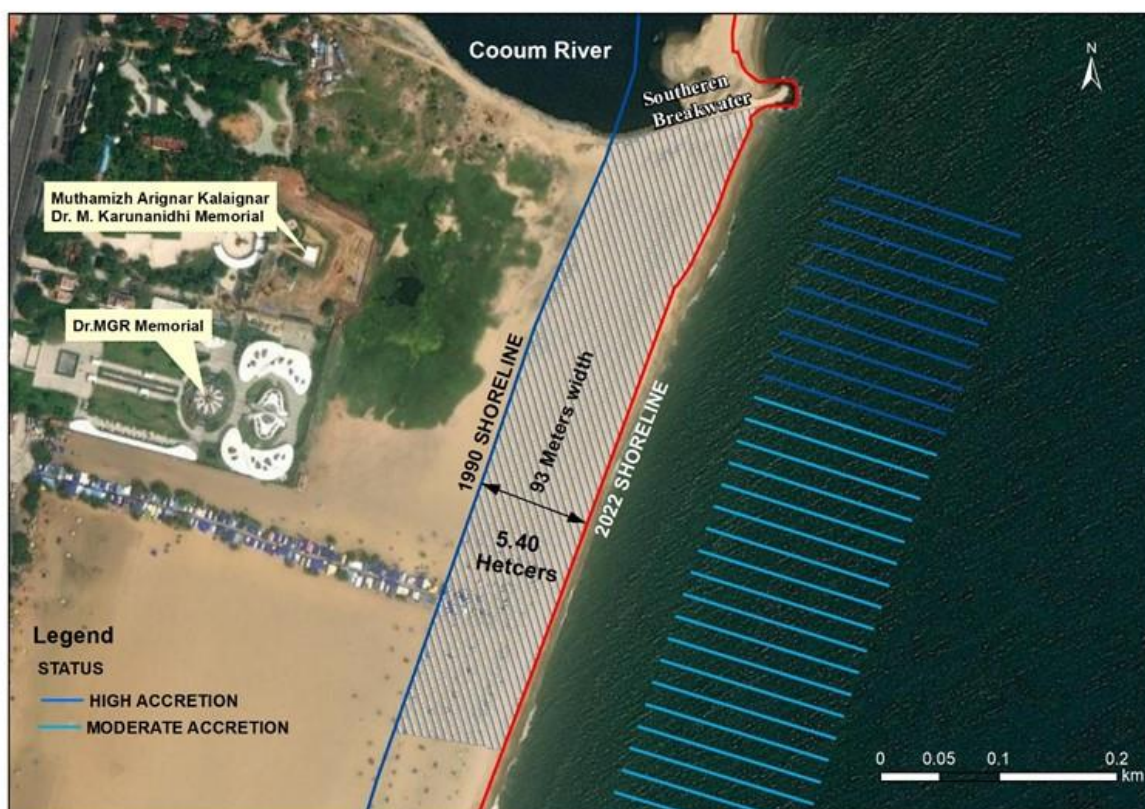
Figure 7: Shoreline position during 1990 and 2022 and status of coast along the location of Proposed Pen Monument
